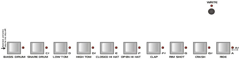
If you now turn the knobs of the selected instrument, all the programmed steps of this track are overwritten with the edits you make. If you want to record dynamic sound scapes, you have to leave the Write Mode by pressing **(Write)** quickly after a successful pattern loop, because on the next loop all steps would be overwritten again.
