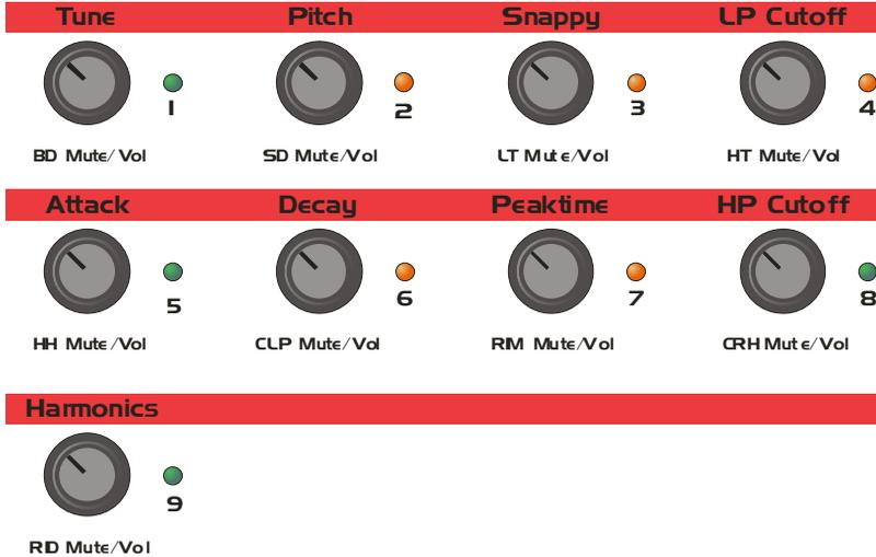
At any time and in any mode, you can mute the instruments by clicking on one of the displayed encoders 1-9. When the instrument is muted, the corresponding LEDs blinks red.
