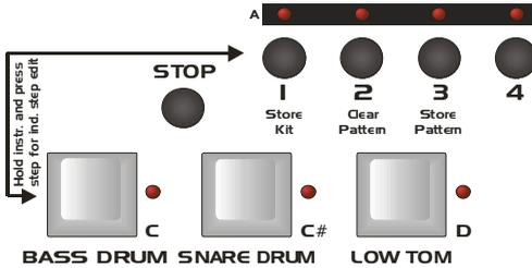
To enter the Individual Step Edit Mode for steps, press and hold the desired **(Instrument)** key and press the desired **(Step)** button(s) at the same time. The selected step LEDs start to flash indicating the Individual Step Edit Mode. The instrument tracks can be switched as used, and the Individual Step Edit steps remain until the Write Mode is left which automatically resets the Individual Step Edit steps.
